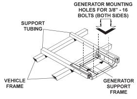
The installer must make certain that the selected location will permit adequate cooling and ventilating airflow to be supplied.
